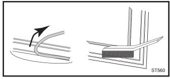
Fig. 33 Remove gasket then clean channel with wire brush.
